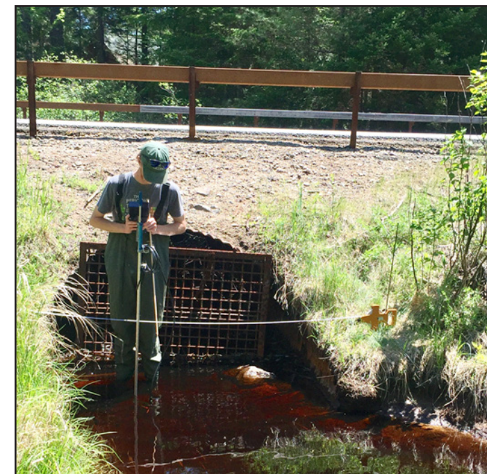
Photo 6. PSCAWI technician, Hunter Favreau measuring the discharge entering Upper Saranac Lake from Brandy Brook.
