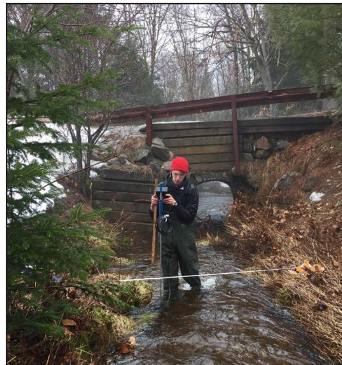
AWI technician, Hunter Favreau, collecting salt loading data from an inlet stream to Blue Mountain Lake. Spring melting conditions, such as the one pictured above, can result in as much as 5,000 Kg/day of chloride entering Blue Mountain Lake from NYS 28/30 (Laxson et al. 2018d).
