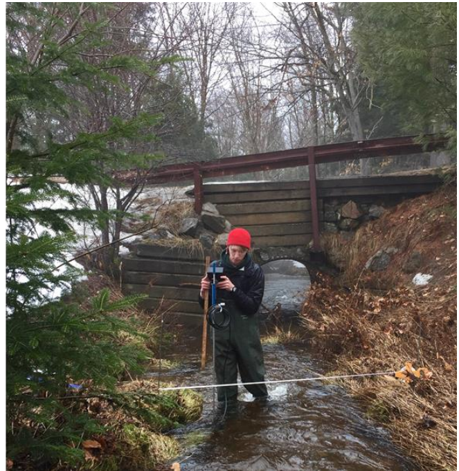
Photo 1. Stream monitoring station at Minnow Brook West (left). AWI Technician measuring stream discharge at Museum Brook (right).
