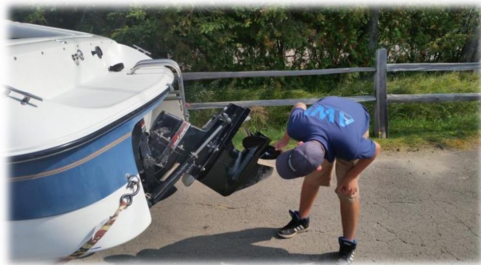
Inspection of the motor’s lower unit is critical to detect hitchhiking organisms.
