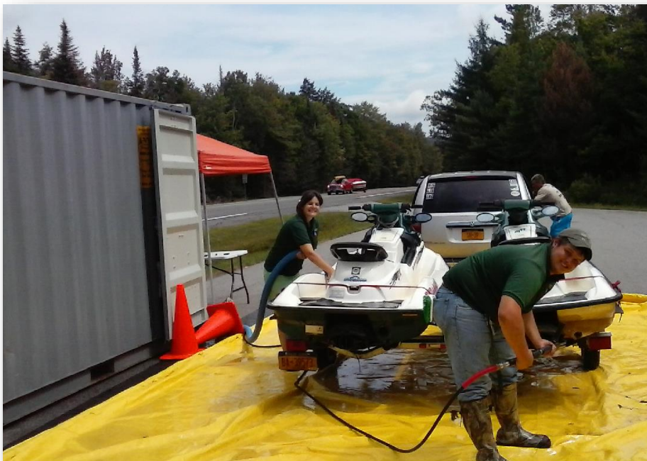
ECOS unit in operation with storage container and wash water mat.
