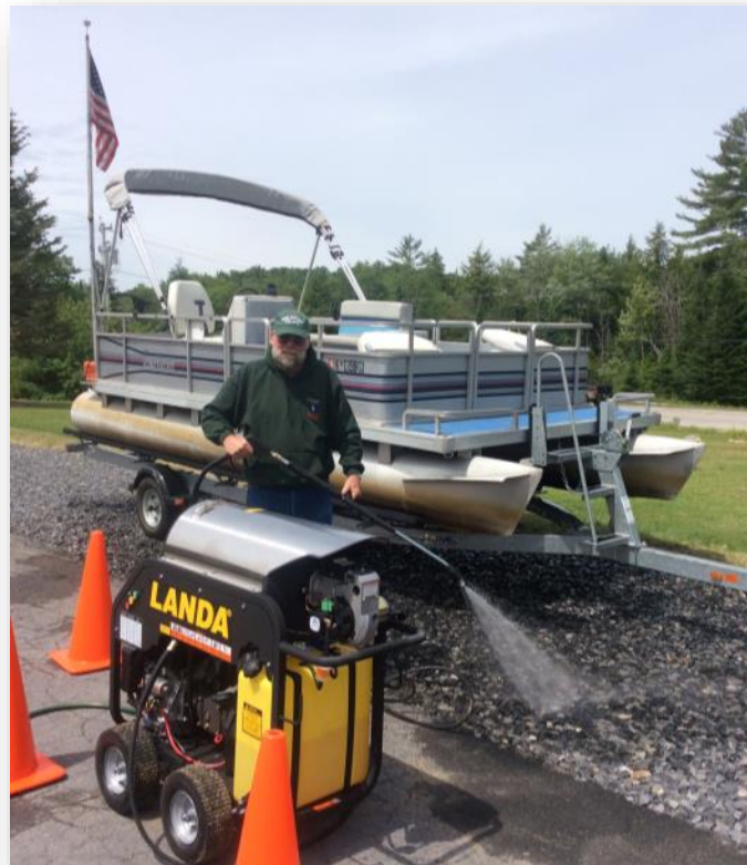
Figure 6. Decontamination station with high pressure, hot water unit and run-off percolation pad.
