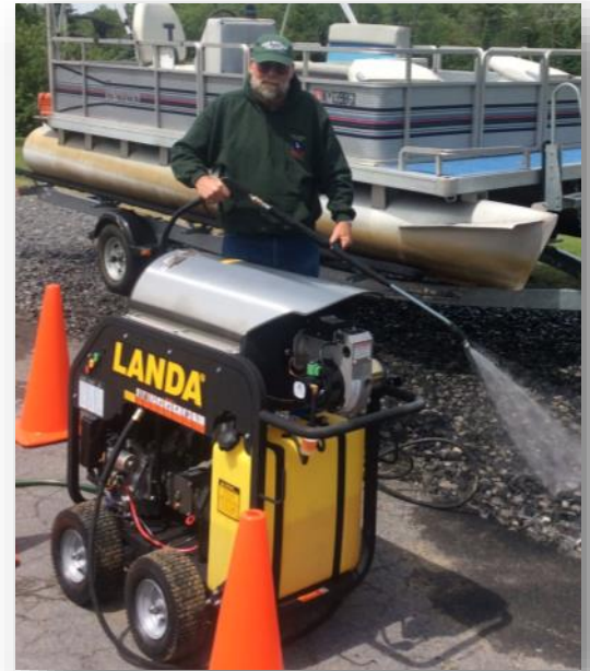
Landa MHC high pressure hot water unit in action.
